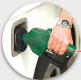
1. The driver inserts the fuel nozzle and the AIM module reads the RFID tag on the nozzle.
