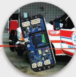
2. The module transmits the tag ID and vehicle data to the Fuel Management Unit (FMU). The FMU activates the dispenser.
